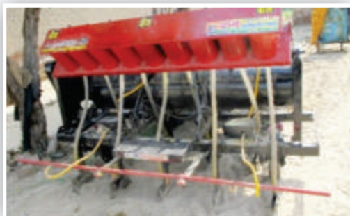
Machine used for sowing of DSR as well as pre-emergence spray
