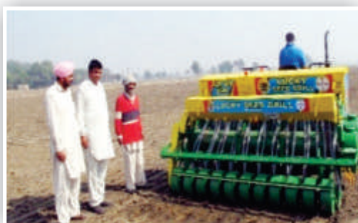
Wheat sowing as well as pre-emergence spray of pyroxasulfone + pendimethalin with lucky seed drill
